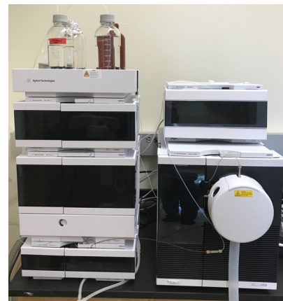
Agilent Liquid Chromatograph – Mass Spectrometer Required by ACS; Used in course work and in student-faculty research Purchased 2018
