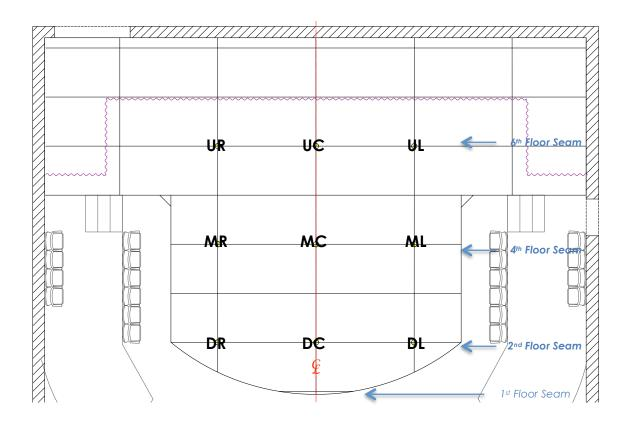
\*Rectangles indicate layout of 4x8 masonite floor boards.
